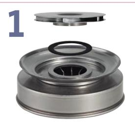
Loss of efficiency has been reduced to an absolute minimum in the impeller stack of the Grundfos CR pumps. This has been achieved for instance by applying a floating seal ring as a perfect seal between the individual chambers.
